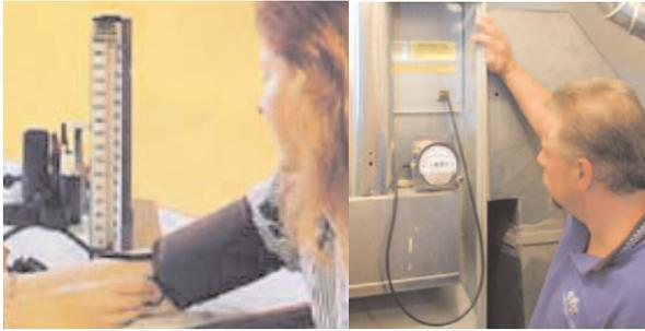
Like blood pressure, Static Pressure is one of the key vital signs of your comfort system. This test helps your contractor identify any significant blockage or leakage.
